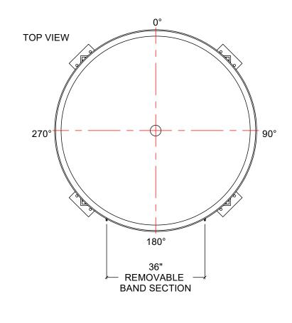
NOTES: 1. TANK IS MANUFACTURED FROM POLYETHYLENE (PE). 2. RATING FOR STORING LIQUIDS WITH A SPECIFIC GRAVITY (DENSITY) OF 1.5SG. (1.9SG OR 2.2SG ALSO AVAILABLE) 3. ALL TANK DIMENSIONS ARE SUBJECT TO A +/-3% TOLERENCE. 4. ALL EXTERNAL PIPING AND ACCESSORIES MUST BE FULLY SUPPORTED AND FLEXIBLE TO AVOID STRESSING THE TANK. 5. FITTING GASKETS AVAILABLE IN EPDM OR VITON.
