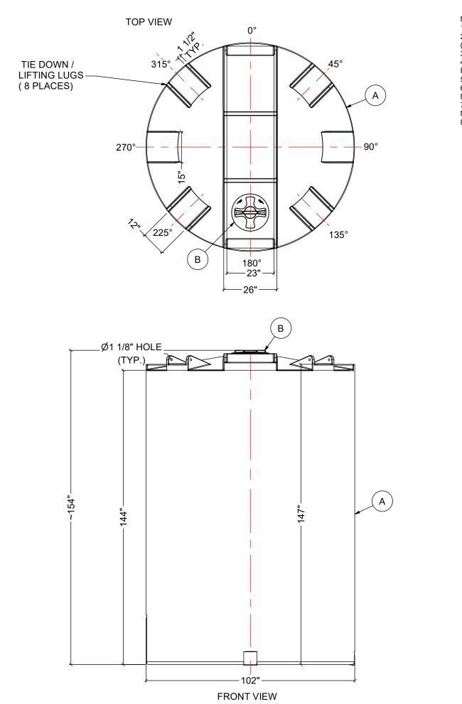
NOTES: 1. TANK IS MANUFACTURED FROM POLYETHYLENE (PE) OR CROSSLINK PE (XLPE). 2. RATING FOR STORING LIQUIDS WITH A SPECIFIC GRAVITY (DENSITY) OF 1.5SG. (1.9SG ALSO AVAILABLE)
