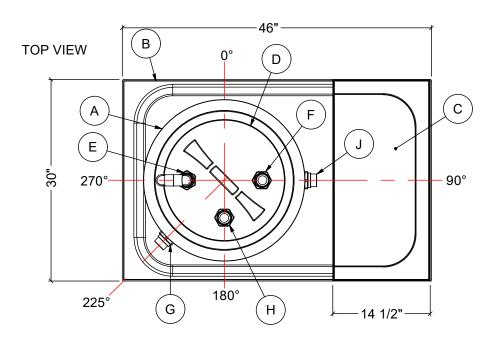
NOTES: 1. ALL TANK DIMENSIONS ARE SUBJECT TO +/-3% TOLERANCE. 2. ALL EXTERNAL PIPING AND ACCESSORIES MUST BE FULLY SUPPORTED TO AVOID STRESSING THE TANK. 3. CONTACT YOUR CHEMICAL SUPPLIER TO ENSURE ALL MATERIALS ARE COMPATIBLE WITH THE PRODUCT YOU INTEND TO STORE.
